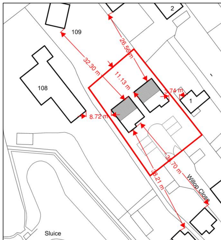
Fig. 9 – Separation distances to existing properties
